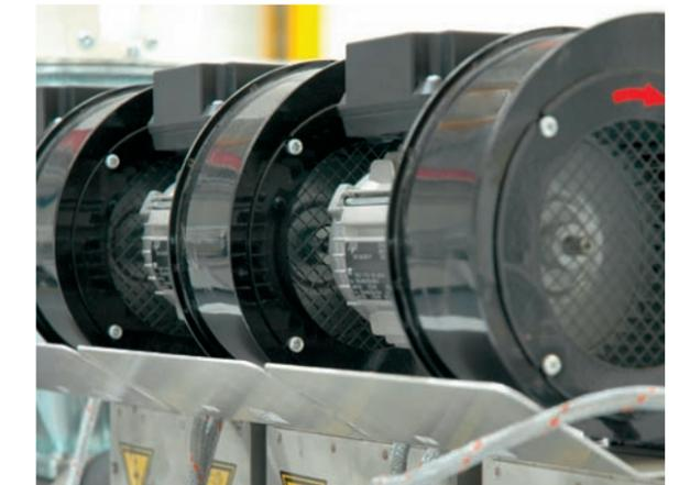
Suitable for all substrates: Seam extruder with individually adjustable heating and cooling zones
