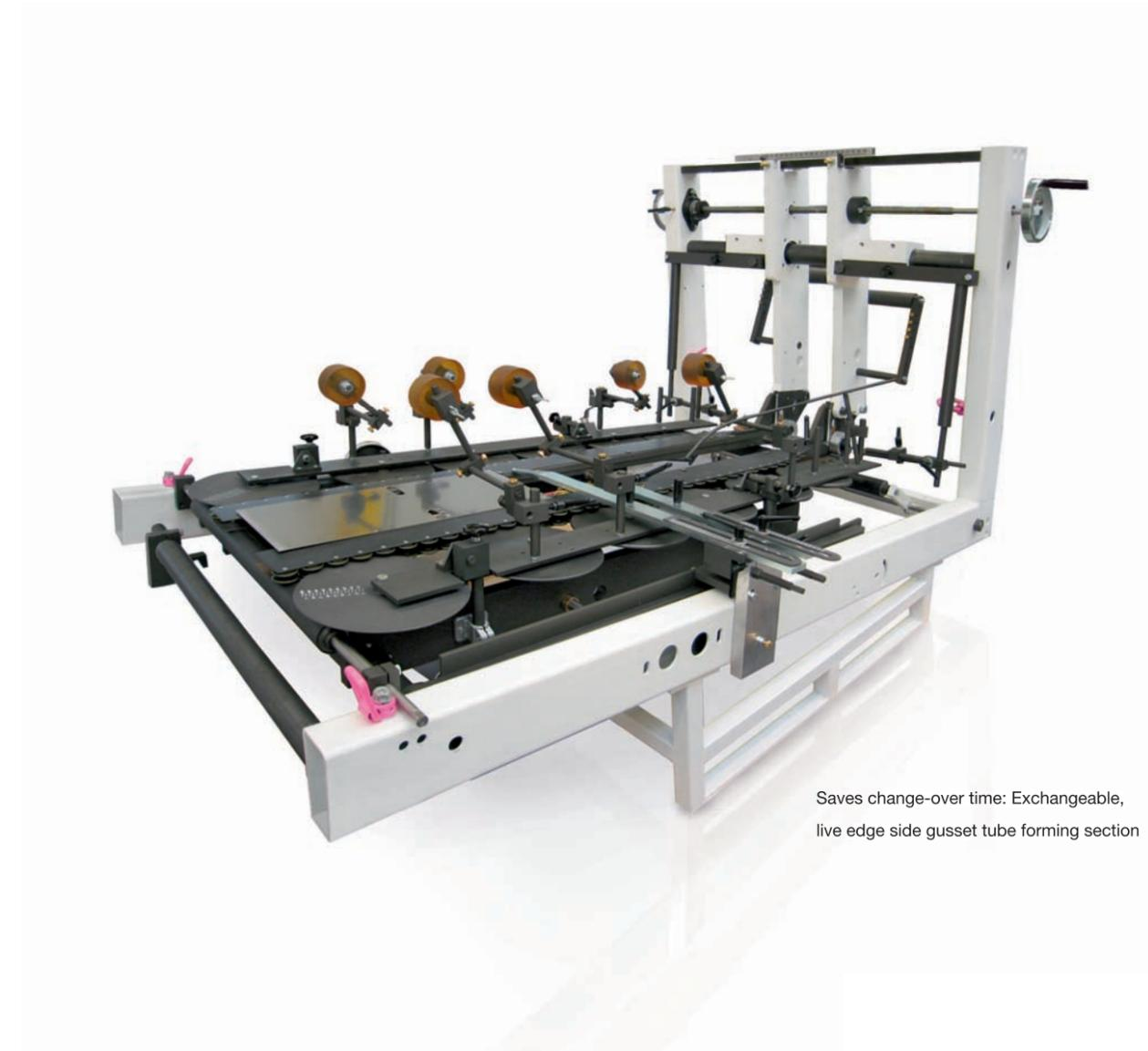
Saves change-over time: Exchangeable, live edge side gusset tube forming section
