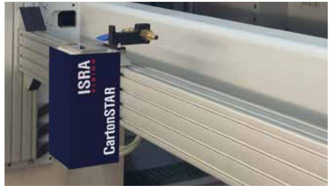
The CartonSTAR inspection system is suitable for examination of post-print of corrugated board, laminating of pre-printed labels on board, pre-print processes of corrugated and solid fiber boxes.
