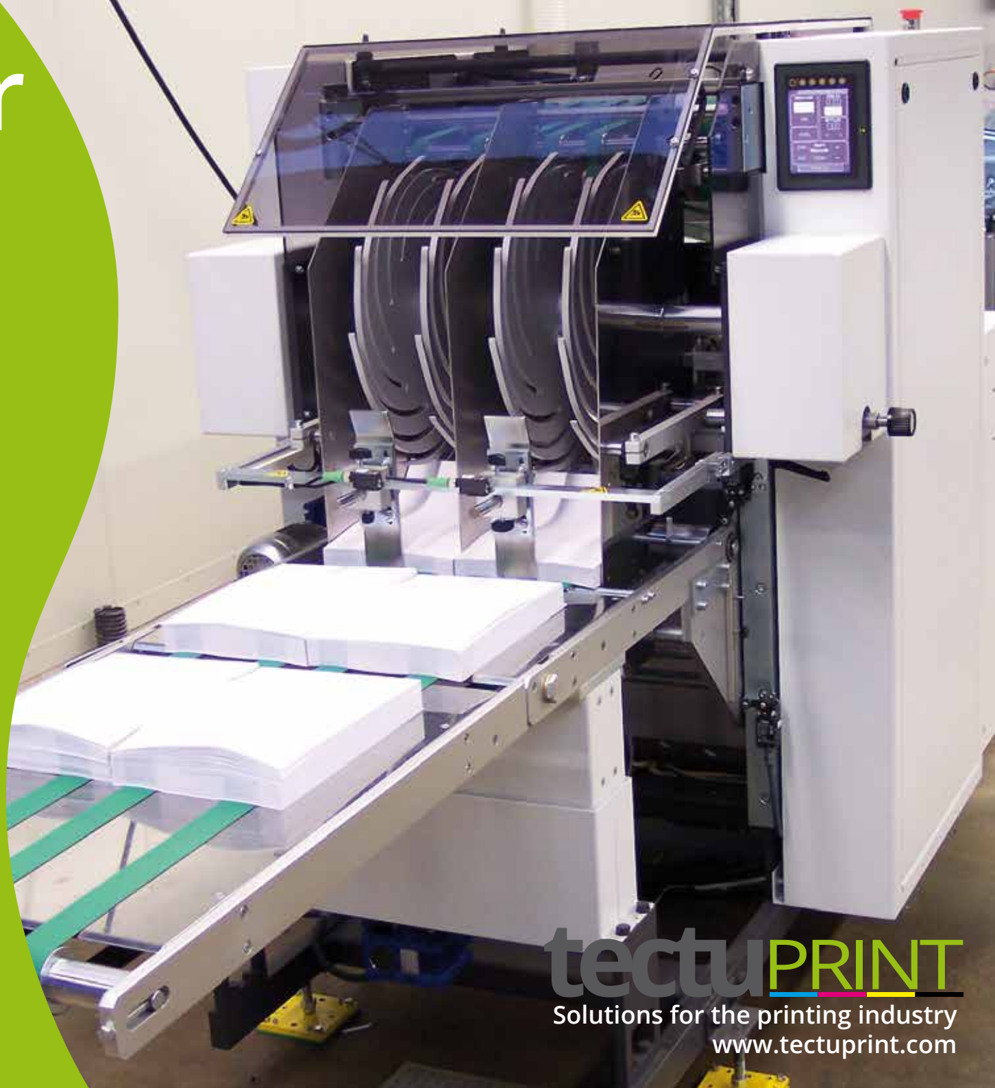
A Sheeter | 1 Infeed belt table | 2 Star wheel | 3 Stacker
