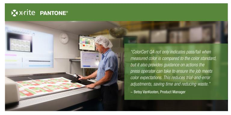
ColorCert QA's BestMatch feature makes it fast and easy for press operators to determine ink density/strength adjustments to correct color on press.
