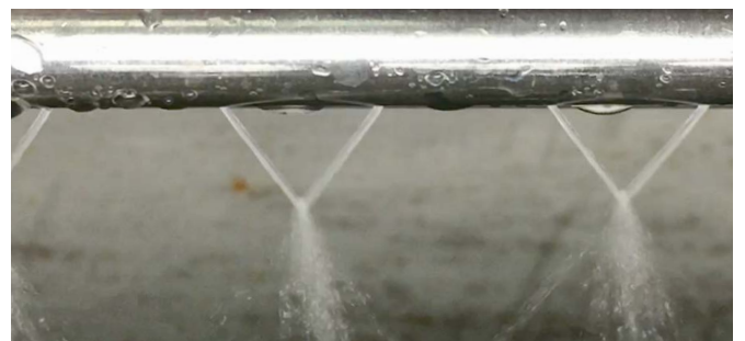
The fluid management system enables efficient cleaning over the full plate width.
