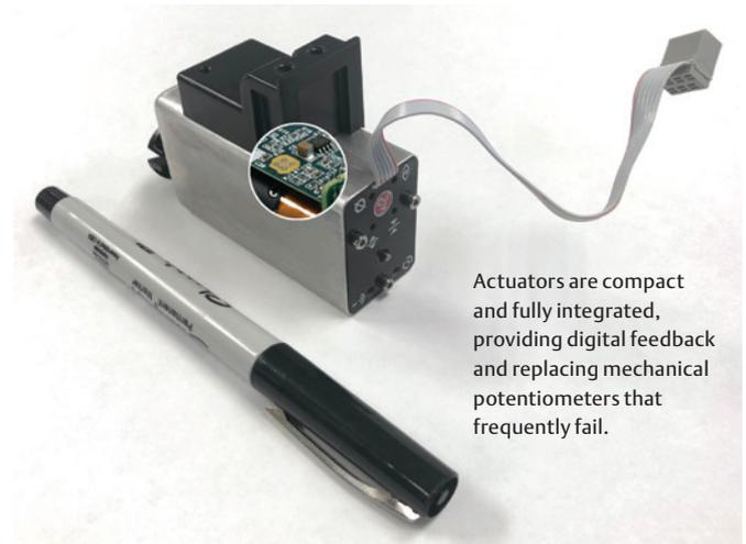
Actuators are compact and fully integrated, providing digital feedback and replacing mechanical potentiometers that frequently fail.
