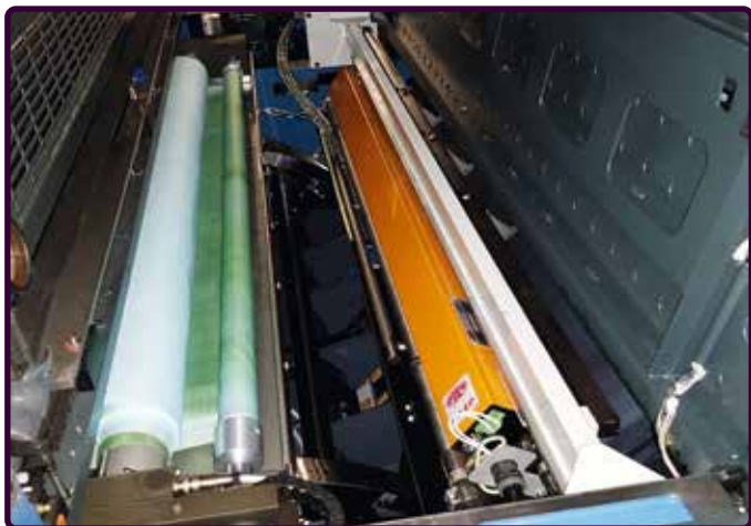
Interdeck G-LED su KBA Metalstar 3 Interdeck G-LED on KBA Metalstar 3
