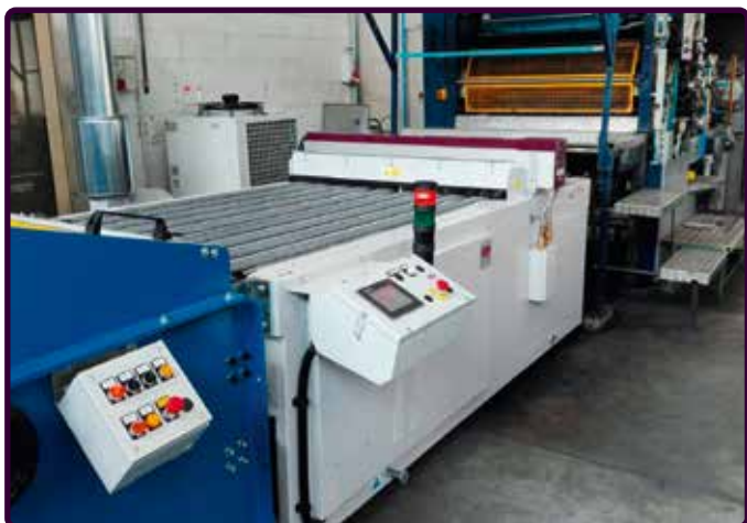
Forno G-LED set-stack in linea a Mailaender 121 Set-stack G-LED dryer in line to Mailaender 121
