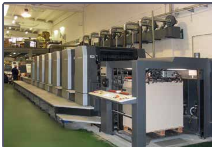
Forno GST/UV su Heidelberg SM CD 102, 6 colori + L GST/UV dryer on 6-colour + Coater Heidelberg SM CD 102
