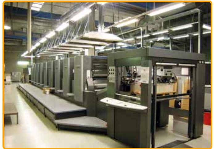
Impianto GST/UV su Heidelberg SM CD 102, 8 colori + LX GST/UV equipment on 8-colour + LX Heidelberg SM CD 102
