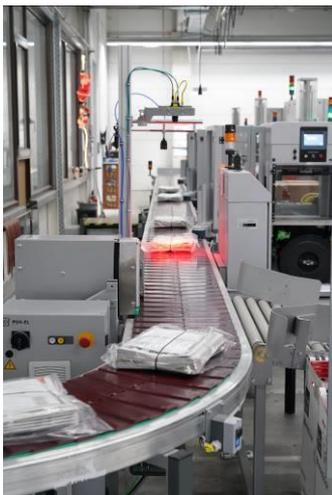
A third Ferag MultiStack compensating stacker has also been added, featuring a state-of-the-art dispatch system for the finished newspaper bundles.
