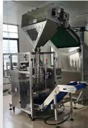
*Scatter and packing machine with conveyor (inline working)
