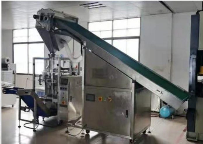
*Scatter and packing machine with conveyor (inline working)
