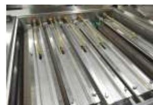
EXCEL-SOLV 3648 is designed as inline high productivity photopolymer plate washing, rinsing and pre-drying equipment, suitable for processing high quality plates up to a maximum size of 920 x 1200 mm.
